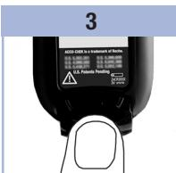
Use your thumb to slide the battery drawer out of the meter.
