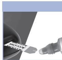
Touch the drop to the **front edge** of the yellow window of the test strip until you see flash.
